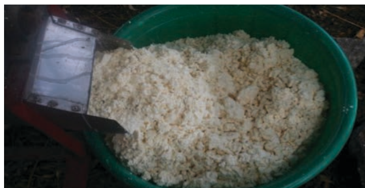
Grating cassava tubers using a grating machine
