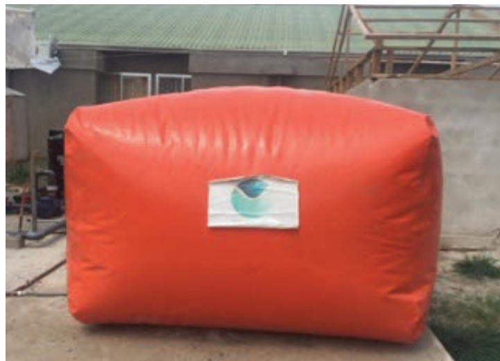
Upgraded biogas (>95% CH 4 ) is collected in a gas bag and used to heat the hybrid dryer for drying cassava grits
