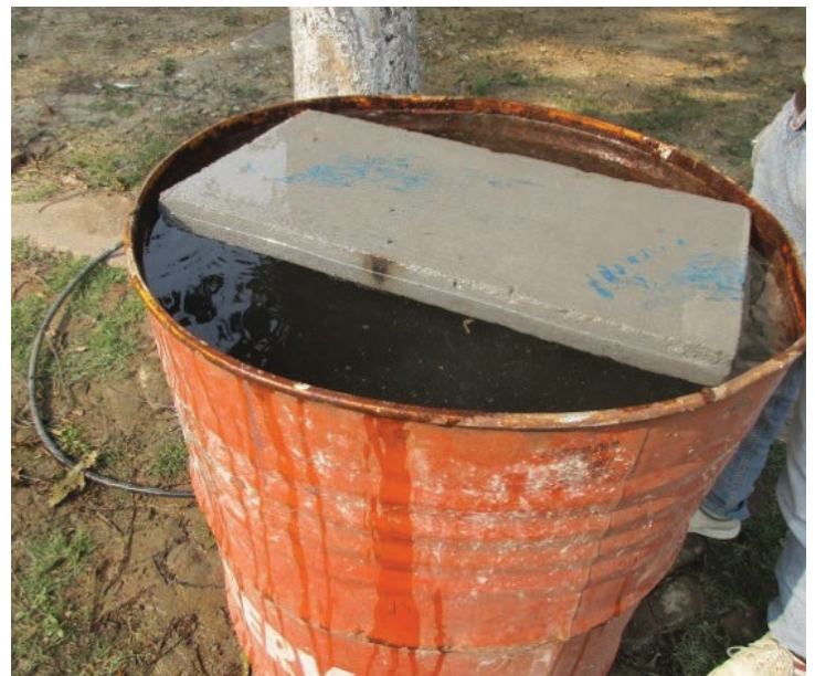
Hydrogen bubbles in the AAC block keeps them afloat
