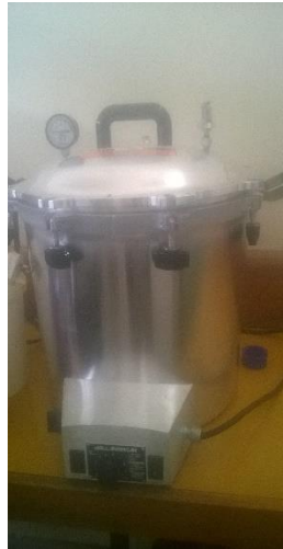
Figure 1: Autoclave, will be used to autoclave prepared food to ensure it is free of pathogens
